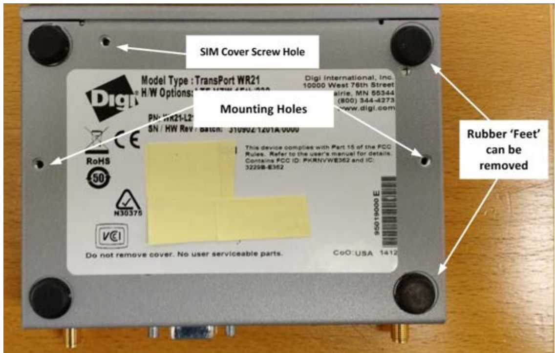
Bottom view of a Digi TransPort WR21.
