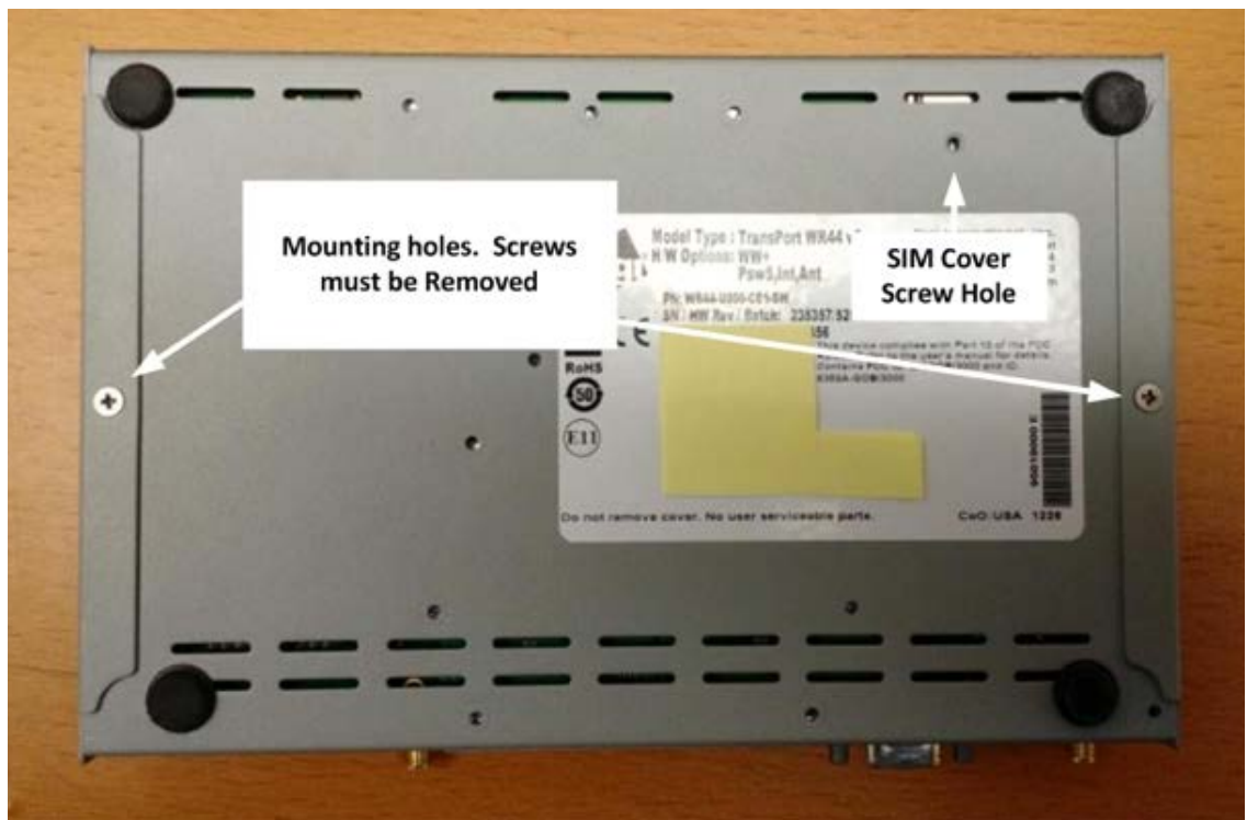
Bottom view of a Digi TransPort WR44.
